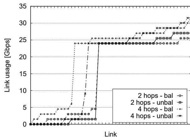
Fig. 5: Link usage of DPP in the network A, balanced and unbalanced, under different hop constraints. Links are sorted from the lowest to the highest usage one.
