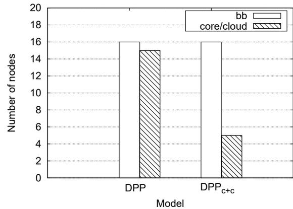
Fig. 4: Number of nodes performing at least one baseband (bb) processing (either L1, L2 or L3), core and cloud functions for the balanced case with 2 hops constraints for DPP and modified  $DPP_{c+c}$  models in network A.
