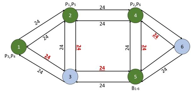
Fig. 7: Outcome of the SPP model in the balanced case for 6 node network and 2 hops as distance constraint. The bandwidth values are in Gbps, red and underlined for the backup path. Dark green color for active nodes.
