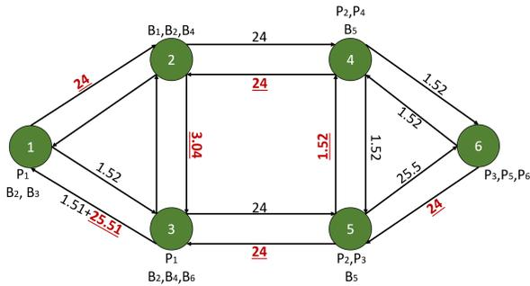
Fig. 6: Outcome of the DPP model in the balanced case for 6 node network and 2 hops as distance constraint. The bandwidth values are in Gbps, red and underlined for the backup path. Dark green color for active nodes.
