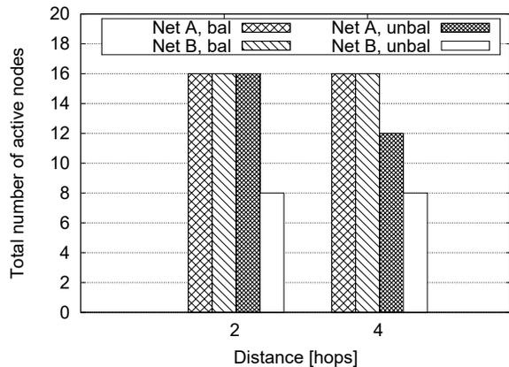
Fig. 3: Active nodes for the networks A and B in the balanced and unbalanced cases with 2 and 4 hops as distance constraint.
