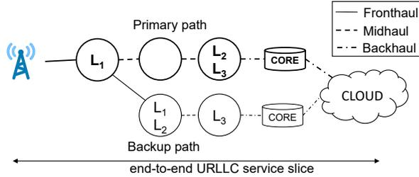
Fig. 1: Example of functional split for URLLC service slice.
