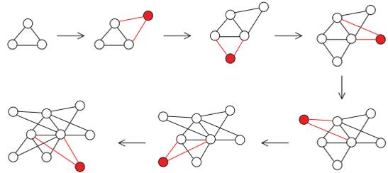
**FIGURE 3.** The generative process of BA scale-free network.
